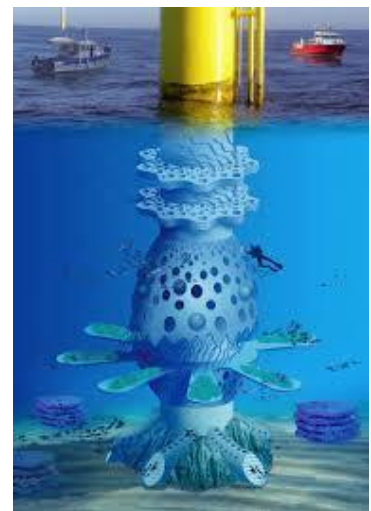
Figure 16 Reef ball shaped ecological foundation of offshore windmill (Building with Nature, 2015).
