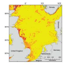
Figure 1: Sediments of the North Sea. Yellow: sand and mud, brown: mixed; orange: coarse (including gravels); red: rocks (EMODnet 2015).
